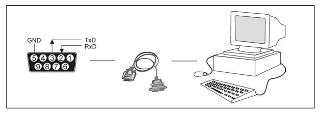
Figure 10 Identification of the interface port pins.
